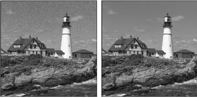
Fig. 2. Two images with identical PSNR of 31.7 dB. The same amount of noise has been added to a rectangular area at the top on the left and at the bottom on the right. The noise is much more visible in the sky than on the rocks and in the water due to strong masking, which PSNR does not take into account.
