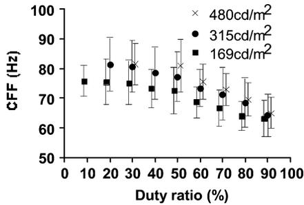
Fig. 2. Mean critical fusion frequency (CFF) and standard deviation plotted against duty ratio. CFF decreased with increasing duty ratio and was higher at higher luminances.
