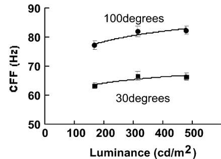
Fig. 4. Screen luminance and critical fusion frequency (CFF) with 30 and 100 degrees FOV. Two regression curves show the CFF prediction equations by Farrell *et al.* [16] CFF was above 60 Hz at 30 degrees FOV and above 80 Hz at high target luminance at 100 degrees FOV.
