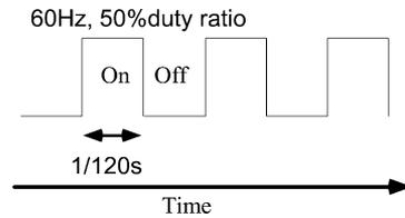
Fig. 5. Intensity of light presented at 60 Hz with a 50% duty ratio. ON and OFF duration were both 1/120 s.
