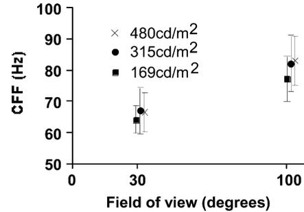
Fig. 3. Mean critical fusion frequency (CFF) and standard deviation plotted against field of view (FOV). With a wide FOV, the CFFs were beyond 80 Hz at high target luminances and were higher than those with a narrow FOV.
