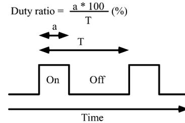
Fig. 1. Duty ratio is defined as the ON duration (a) as a proportion of the ON+OFF duration (T).
