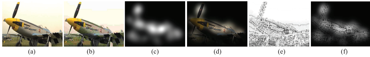
Figure 11 (Color online) An illustration of saliency weighted IQA. (a) Reference image; (b) distorted image; (c) saliency; (d) saliency-weighted image; (e) SSIM; (f) saliency-weighted SSIM.
