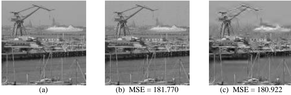
Fig. 2. Harbor image altered with two types of distortions: (a) reference image; (b) white Gaussian noise; (c) quantization of the LH subbands of a 5-level DWT of the image with equal distortion contrast at each scale. All images are extracted from [51].
